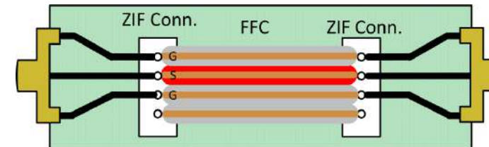
Balanced measurement (differential)
