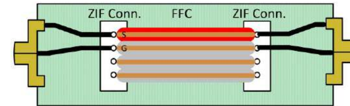
Unbalanced measurement (single)
