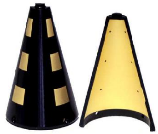
12-element conical phased array antenna for discrete communications in the 5,2 GHz band. ISL, DGA
