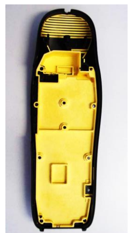
PMR, BT antennas and integrated shielding in one part Airbus D&S, Radiall
