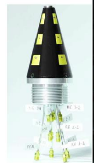
12-element conical phased array antenna for discrete communications in the 5,2 GHz band. ISL, DGA
