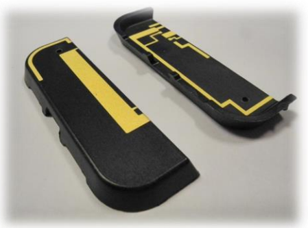
LTE antennas mobile communications ST Microelectronics
