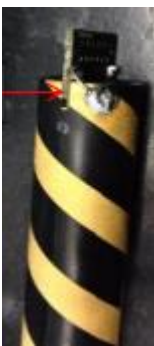
8 MHz double helix antenna for agriculture sensors LAAS
