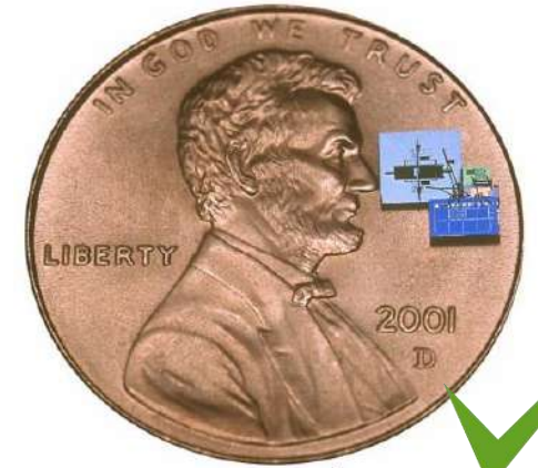
Berkeley « Smart-Dust » - 2002 16 mm 3 autonomous solar- powered sensor node
