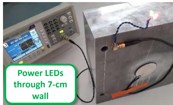
Acoustic WPT demo through thick wall
