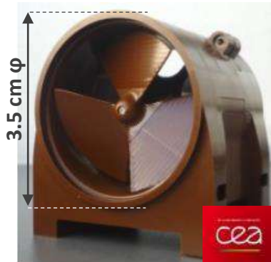
250°C compliant \mu turbine for aeronautic env.
