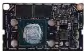
JETSON NANO 5 - 10W 0.5 TFLOPS (FP16) 45mm x 70mm $129
