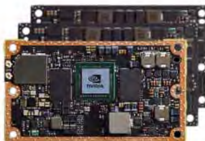
JETSON TX2 7 - 15W 1.3 TFLOPS (FP16) 50mm x 87mm $399 - $749
