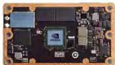
JETSON TX2 4GB 7 - 15W 1.3 TFLOPS (FP16) 50mm x 87mm $249
