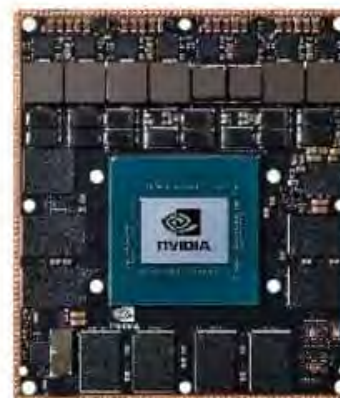
JETSON AGX XAVIER 8GB 10 - 30W 5.5 TOPS (FP16) 11 TOPS (INT8) 100mm x 87mm $599
